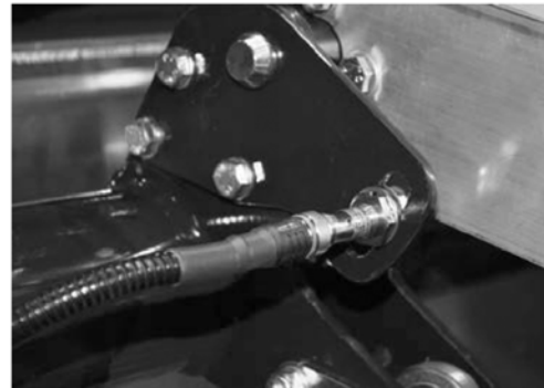
Sensor (E4) for sweeper position, backward
