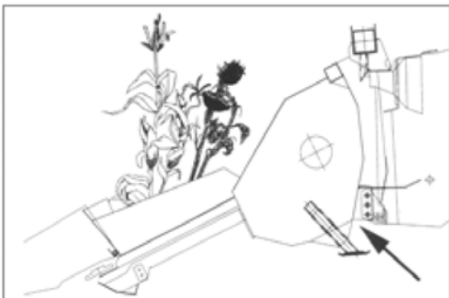
Support legs in transport position
